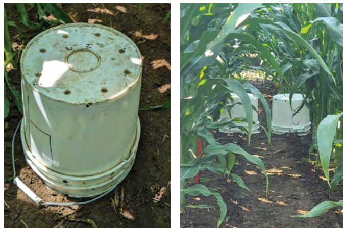
Figure 1. Dositube chambers in a corn field for measuring ammonia volatilization loss from a sidedress nitrogen application.
