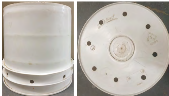
Figure 2. Dositube chamber showing holes drilled through the bottom and around the lip of the bucket
