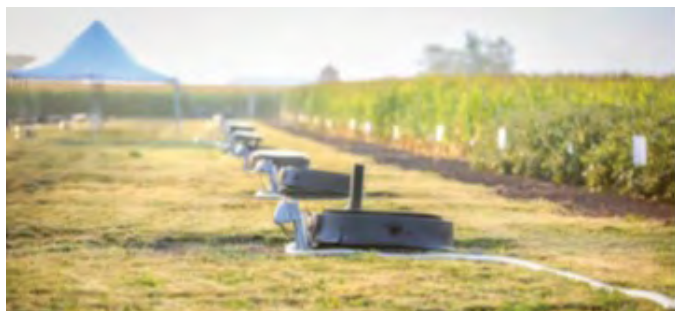
Figure 1. Field research was conducted in 2023 to test the effect of Instinct NXTGEN nitrogen stabilizer on nitrogen loss through tile drainage at a field research site with drainage infrastructure in place to allow sampling of nitrogen content in drainage water.
