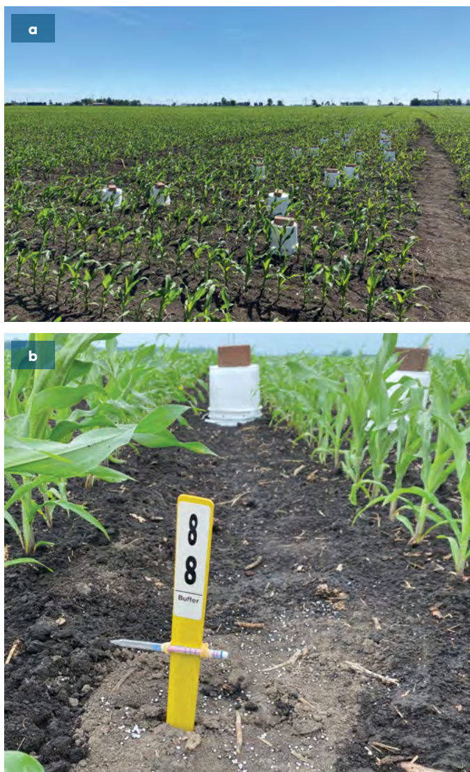
Figure 2a. Overview of the various treatments with dositubes and buckets measuring volatilization. Figure 2b. A dositube connected to a wooden stake (foreground) and the bucket that is placed over the wooden stake to define the measurement area (background). Photo taken near Windfall, IN, in 2021 by Rebecca Hensley.
