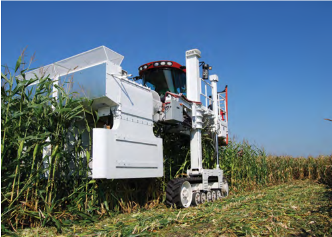
Figure 6. Corteva Agriscience's Boreas wind machine creates winds that can exceed 100 mph to test for standability in corn hybrids.
