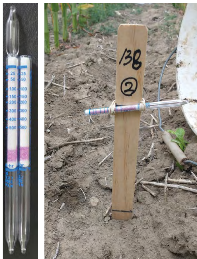
Figure 3. Left: Dositubes used for measuring ammonia volatilization, showing where to break the dositube to begin measurement. Right: A dositube attached to a wooden stake with the open end angled slightly downward.
