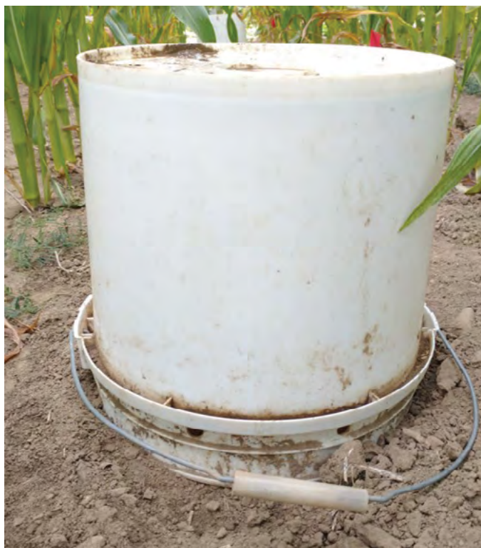
Figure 4. A correctly installed dositube chamber with no gaps between the bucket lip and the soil.
